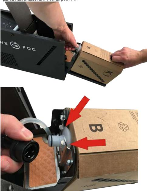
• Check container slips behind the edge of the fluid container assembly.
