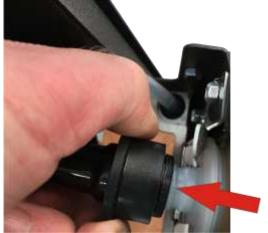
• A small amount of fluid will remain inside the connector, pour out drops onto the cellulose cloth below the connector. Replace cloth when necessary.
